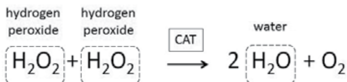
Reaction 10. Catalytic reaction of the enzyme catalase on hydrogen peroxide
