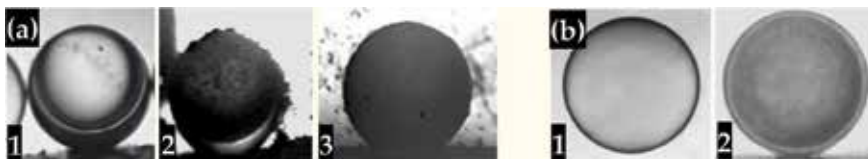
Figure 16. Different protective coatings. In (a): double protection “Pd-coating of 150 Å thick and cryogenic O 2 -coating”: 1—1.2-mm CH-shell at 14.6 K before the experiment (liquid H 2 inside as temperature indicator), 2—in the top part of the shell (from the outside), there is a solid deposit of oxygen ( T_{tp} = 54.3 K), 3—after operation of the piezoelectric vibrator [22], the oxygen snow becomes redistributed onto the outer shell surface; in (b): single protection “Pt/Pd-coating of 200 Å thick”: 1—1.5-mm CH-shell before the experiment, 2—cryogenic target at 5.0 K with a uniform D 2 layer of 50 \mu m fabricated by the FST-layering method.
