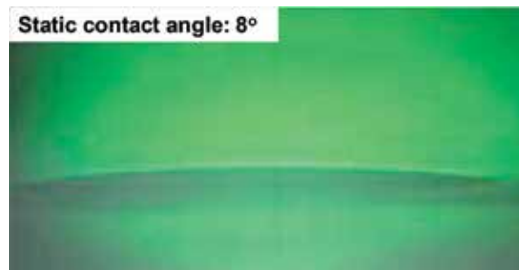
Figure 25. Modification of hydrophilic surface to have superhydrophilic state by laser nanotexturing.
