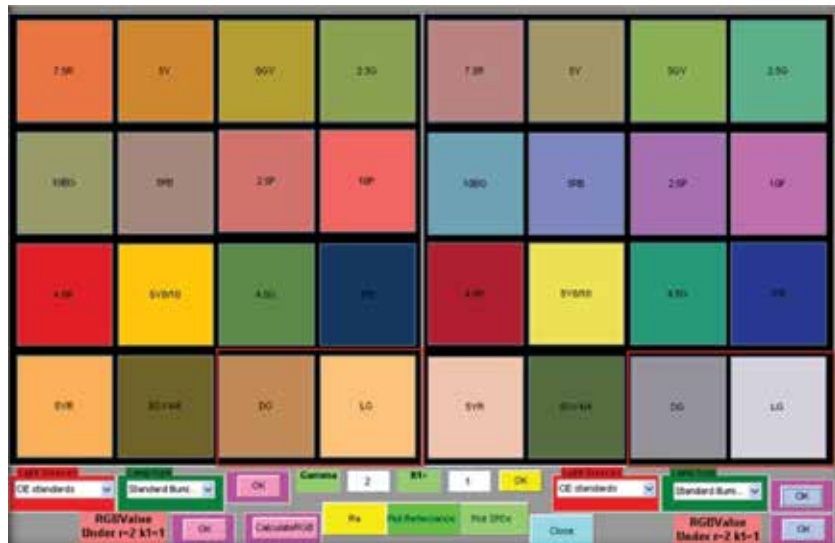
Figure 5. Main display window of the VIS showing illuminant a (left) and D65 (right).
