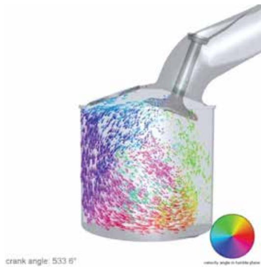
Figure 6. Pathlets visualizing tumble motion of flow. Image courtesy of Garth et al. [6].
