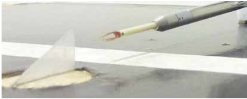
Figure 17. Fin-type vortex generator, with a hot wire anemometer downwards.
