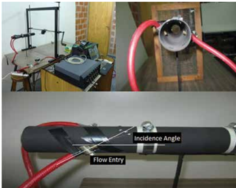
Figure 13. Experimental set-up for longitudinal vortex generation.
