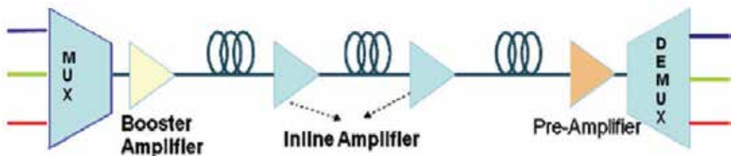
Figure 3. A simple WDM optical network, where a number of transmitted channels are combined using a WDM multiplexer (MUX), amplified using a booster amplifier before being launched into the transmission fiber, re-amplified every 80–120 km using in-line amplifiers, and finally preamplified before being demultiplexed and received [1].
