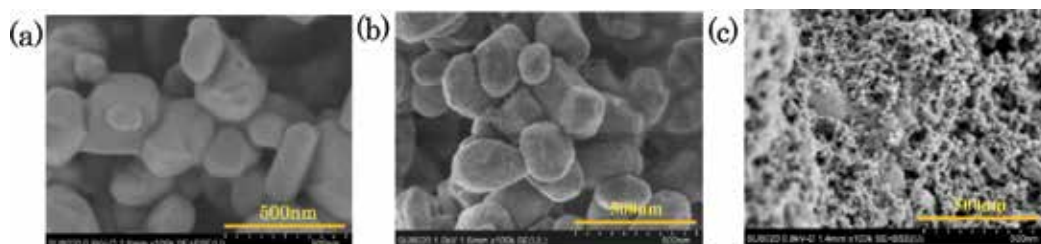
Figure 16. FE-SEM images of titanium oxide particles (a) as-received, (b) after WJ processing, (c) after MFC processing ( \times 100,000 ).
