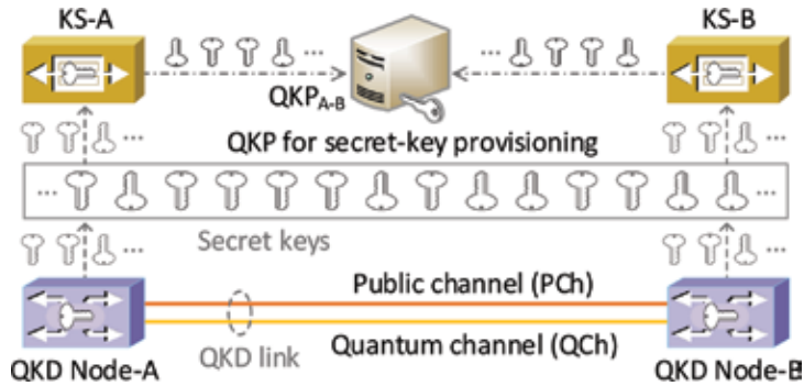
Figure 3. An example of QKP for secret key provisioning between Node-A and Node-B.
