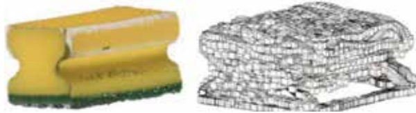
Figure 5. Object representation using the probabilistic volumetric map: sponge and its computed map.
