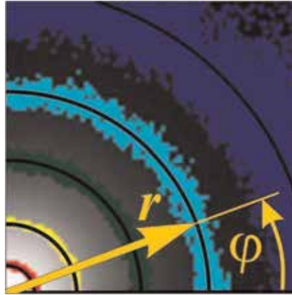
Figure 2. Raw data processing scheme. Averaging the temperatures from a set of pixels located at the same distance r in a fragment of last frame from Figure 1 .
