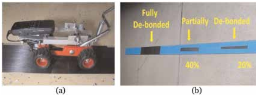
Figure 3. (a) Mobile impact machine and (b) laboratory CFRP test plate.
