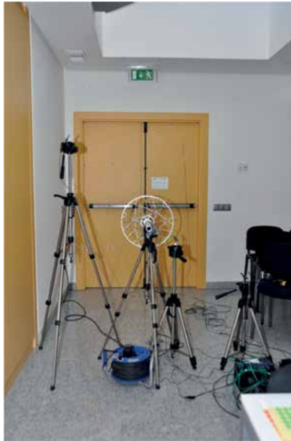
Figure 3. Example of the beamforming measurement layout.
