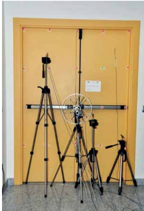
Figure 4. Example of the SONAH measurement layout.
