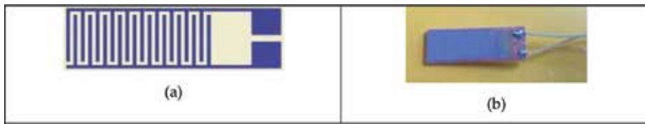
Figure 21. The NO 2 gas sensing element structure (a) PCB substrate with interdigitated Ag array electrode; (b) the sensing element made with PCB substrate and sensitive material deposited on surface electrode.
