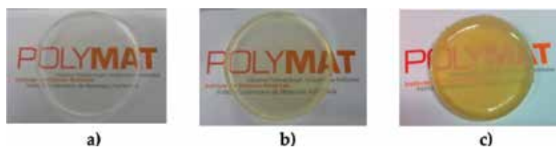
Figure 5. Picture of films cast at room temperature for different CeO 2 loadings: (a) 0% CeO 2 , (b) 1% CeO 2 and (c) 5% CeO 2 .
