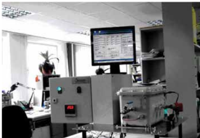
Figure 4. The testing gas sensor installation.
