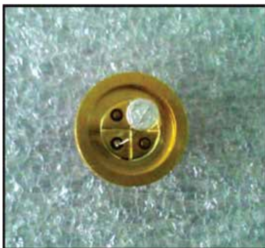
Figure 1. Image of the CO 2 sensor made with mixed oxides CeO 2 -Nb 2 O 5 sensitive material.
