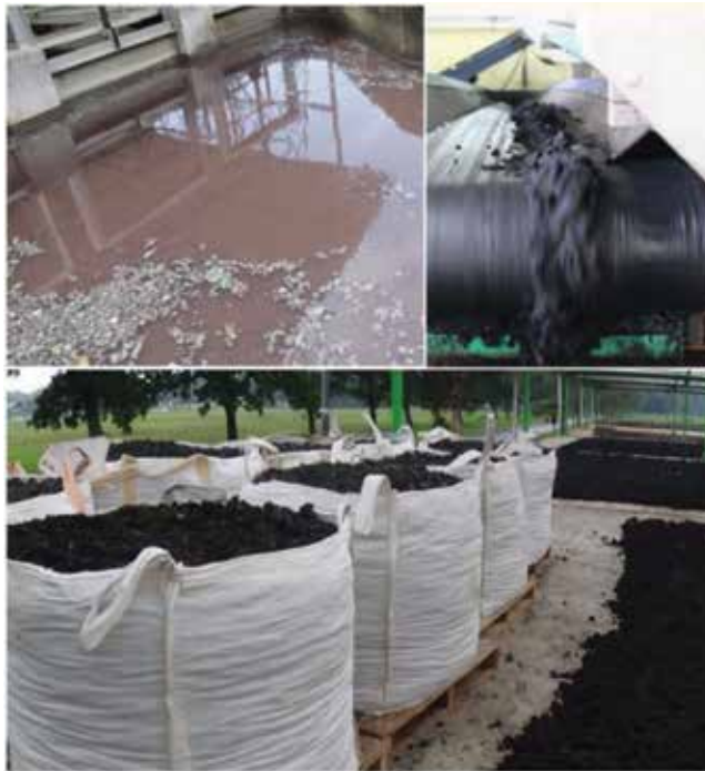
Figure 2. Treated industrial sludge in Jababeka's wastewater treatment facility. (Source: Kurniawan et al.).
