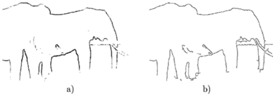
Figure 14. Edge detection for the benchmark image with noise: (a) memristive grid at t = 19.65 ms and (b) Canny's method [2] for a threshold 0.443.
