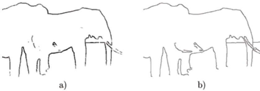
Figure 11. Edge detection: (a) memristive grid at t = 20.45 ms, (b) Canny's method [2] for a threshold 0.422.
