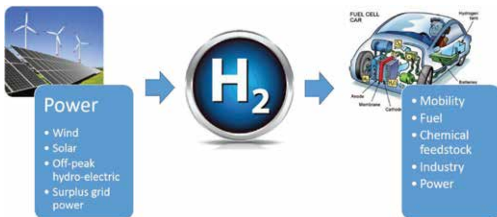
Figure 1. Schematic diagram of power-to-gas strategy.
