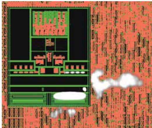
Figure 10. An example of array I/O and latch-up propagation in the core circuitry.
