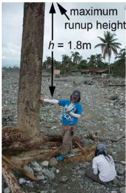
Figure 6. Data used to reconstruct the velocity of the debris flow that destroyed Andap. The woman is pointing at the flow level before run-up. Remnants of Andap are in the background; the yellow sign commemorates all the victims by name.
