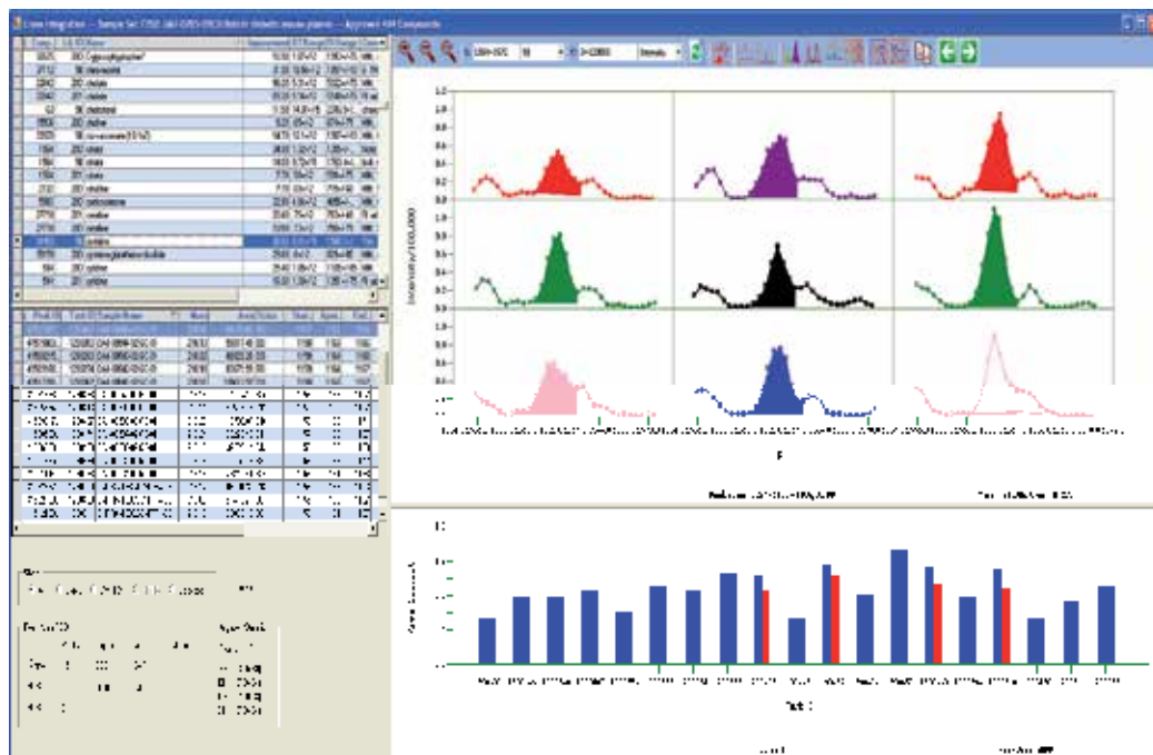
Fig. 7. Graphical View of Peak Integration for an Identified Metabolite: Identified metabolites (200~600) in the specified sample set (Upper Left); Quantitation peaks for selected metabolite in the samples in the sample set (Middle Left); Type of samples and Information about the sample peaks (Lower Left); Peak chromatograms (Upper Right); Sample peak area (blue for original integration and red for re-integrated (Lower Right)).
