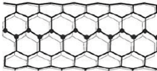
Figure 2. Fluorinated nanotube F-(n, n) (dots denotes the positions of Fluorine atoms of Fluorine atoms that are covalently bonded to C atoms).
