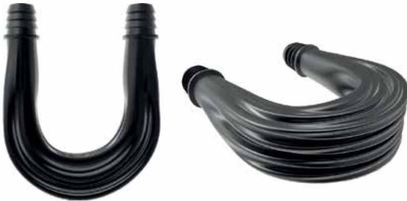
Figure 22. A computer-aided designed curved heat exchanger. Its geometry bases on FASS.
