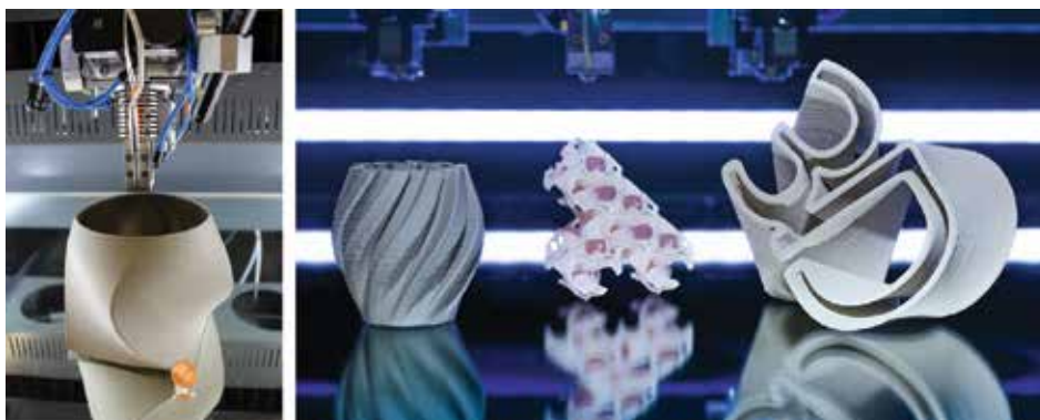
Figure 20. Different ceramic demonstrators additively manufactured by FFF; left: SiC (green state); right: various ceramics (sintered state).
