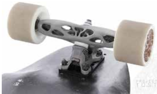
Figure 16. Complexly designed skateboard trunk manufactured with LBM.
