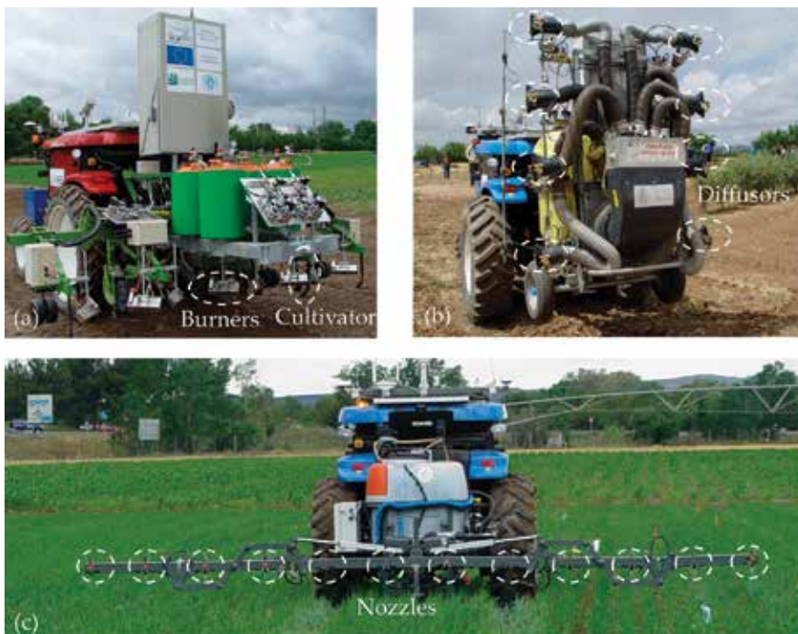
Figure 6. Implements working: (a) thermal and row cultivator, (b) canopy sprayer and (c) patch sprayer.
