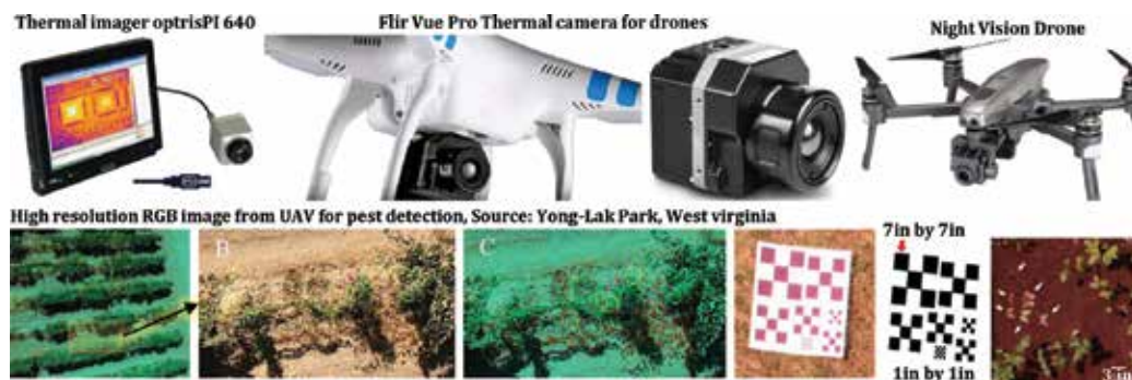
Figure 8. Thermal camera and night vision (top row figures) and high-resolution RGB images approach (bottom row figures) for UAV based pest monitoring in oil palm plantations.
