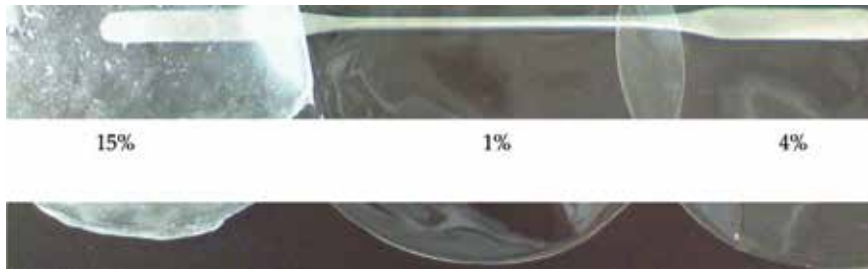
Figure 1. Appearance of PVOH films with different concentrations of inclusion complex. Films elaborated at concentrations of 1, 4, and 15% of EO by process A (molar ratio \beta -CD: AO 1:10).
