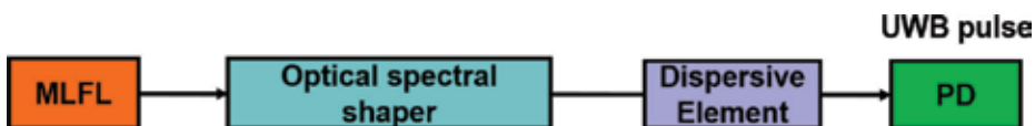
Figure 7. The block diagram of a UWB-IR generation system based on optical spectral shaping and frequency-to-time mapping. MLFL, mode-locked fiber laser.
