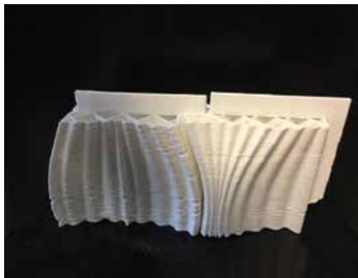
Figure 16. G. Rossi at ACTLab, 3D printed interlocking structure (credits Politecnico di Milano University).
