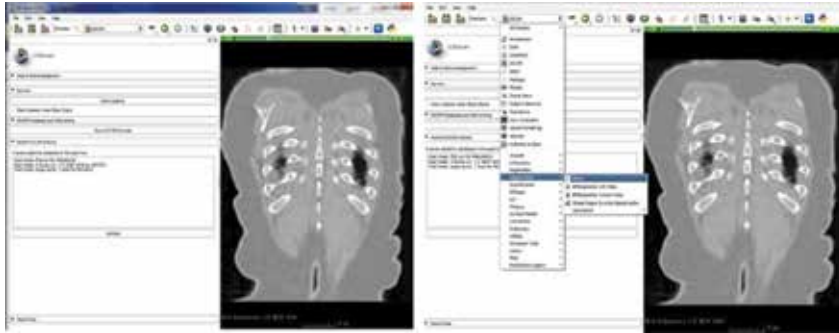
Figure 6. Steps 5–6: Finding the correct slice and open the segmentation editor.
