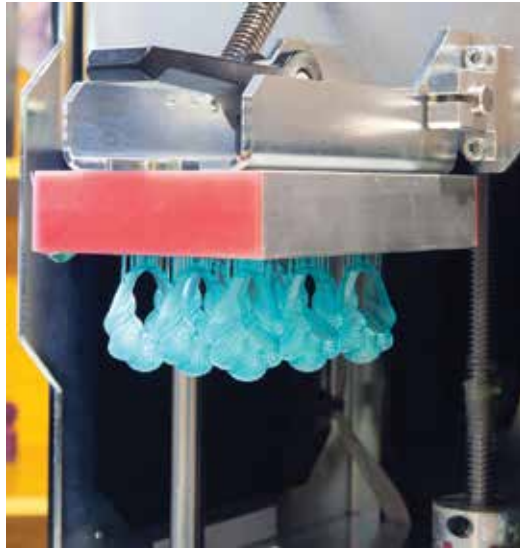
Figure 4. Example of SLA production ( https://tinyurl.com/yal2wluv ).
