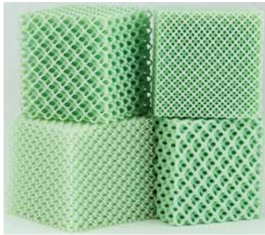
Figure 6. Carbon 3D printed lattice structure ( https://tinyurl.com/y8n472bs ).
