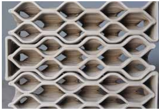
Figure 14. Clay printed modular structure ( https://tinyurl.com/yb62v3cz ).
