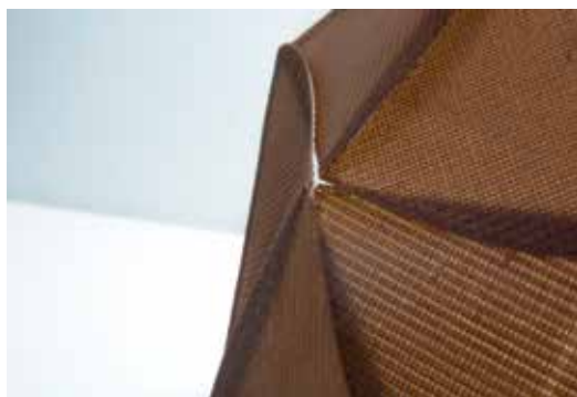
Figure 23. Correa et al., 4D printed adaptive component: when closed ( https://tinyurl.com/yd7dy728 ).
