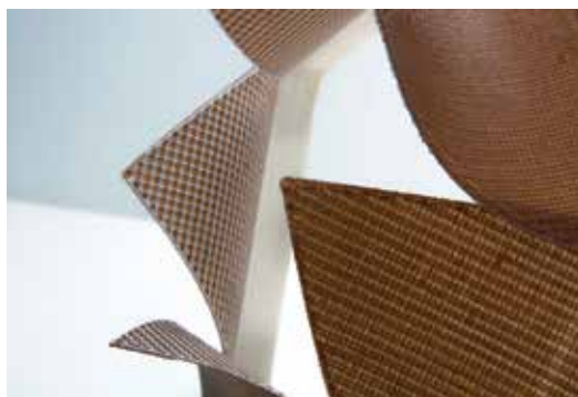
Figure 24. Correa et al., 4D printed adaptive component: when open ( https://tinyurl.com/yd7dy728 ).
