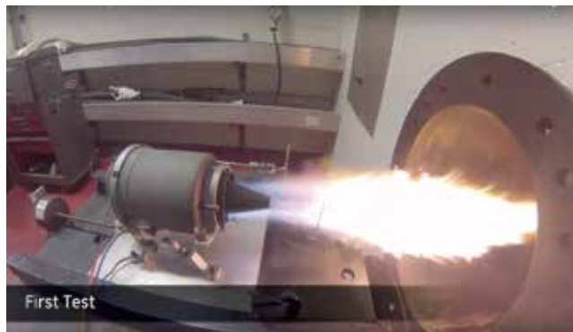
Figure 17. GE fully 3D printed working engine prototype ( https://tinyurl.com/y85355af ).
