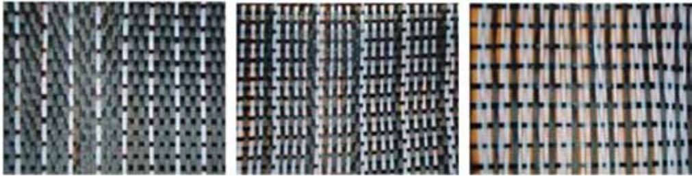
Figure 10. Various geotextiles for antireflective crack propagation.
