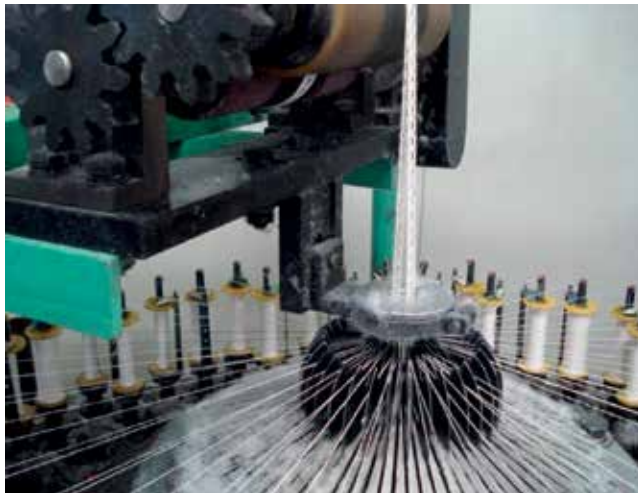
Figure 12. Accumulation of broken fibers at fell point due to beatup knife abrasion.
