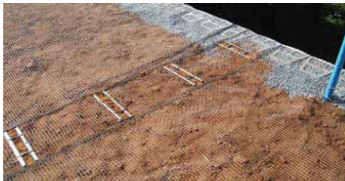
Figure 7. Load cells positioned along the reinforcement [21].
