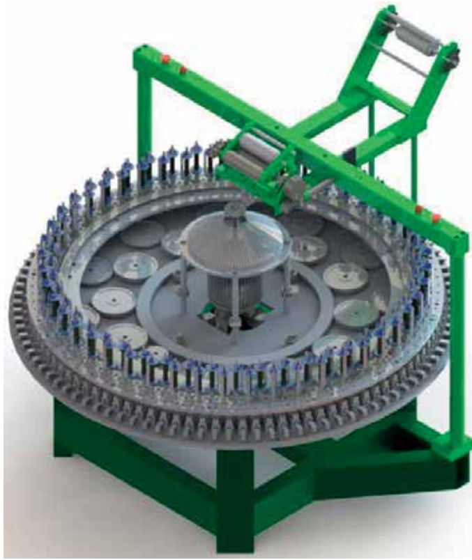
Figure 5. CAD drawing of modern lace braiding machine.
