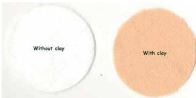
Figure 16. Nonwoven geotextiles with/without nano-clay.
