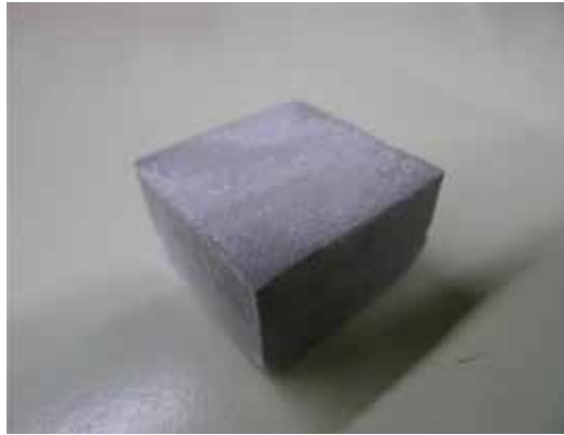
Figure 4. Magnesium hydride (the external size of 35 × 35 × 17 millimeter, Bio-Coke Ltd. Japan).
