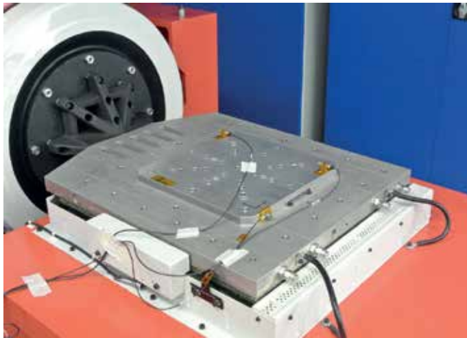
Figure 4. Interface adapter mounted on the shaker slip table.
