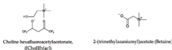
Figure 2. Molecule structures of the extractants applied in HLE for metal ion extraction.
