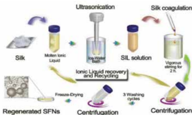
Figure 7. Scheme of the overall process of SF dissolution, using ILs and ultrasonication, and consequent SFNs preparation from SIL solutions. From Ref. [23] with permission of Wiley Online Library.
