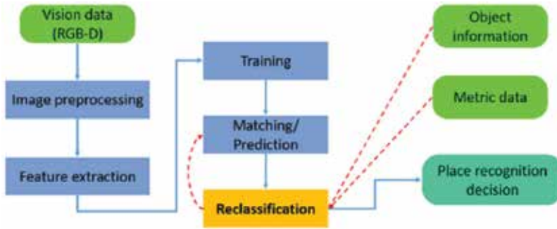
Figure 11. Schematic of a general scene recognition model. Vision data are the initial input of the recognition model. Then, the metric data and object information can be included into the model to update the final outcome of the possible place where the robot can be.
