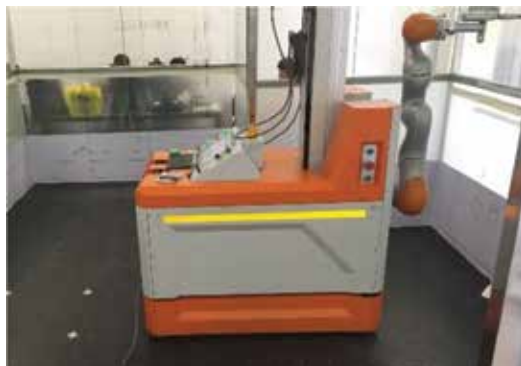
Figure 24. MoMaCo (mobile manipulator in construction).
