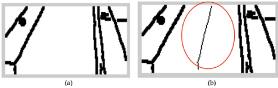
Figure 8. Image sequences processing where no roundabout can be detected using LS, (a) image from preprocessing and processing step, and (b) applying the LS (continues line in the middle).
