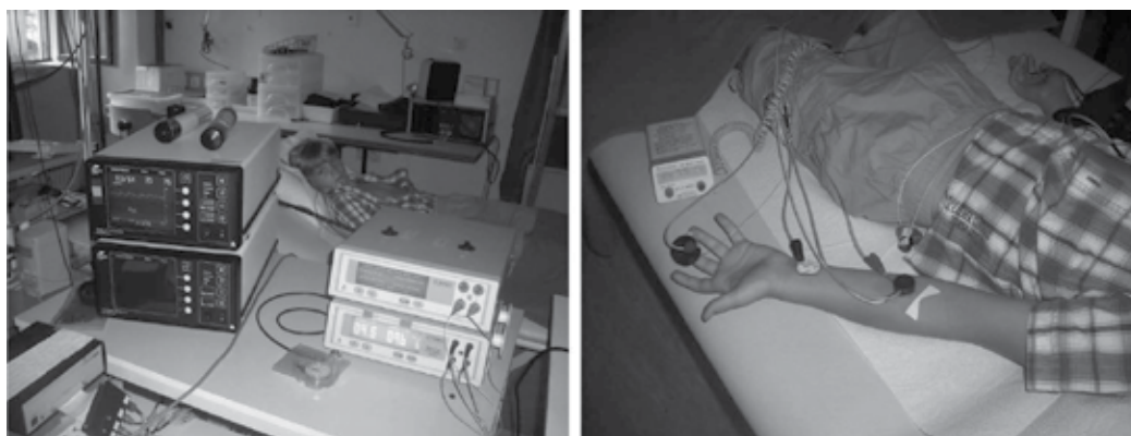
Fig. 2. A typical equipment for assessing skin microcirculation: Laser Doppler flowmeter (LDF, Perimed), the device to register blood pressure in the finger artery (Finapress, Ohmeda), and the transducer for a simultaneous transmission of the digital signals to the computer (left-hand). A typical position of the LDF probes: a standard LD probe (placed on the finger pulp, i.e. representative of glabrous site) and an iontophoretic delivery LD probe (placed on the volar forearm, i.e., representative of nonglabrous area) combined with the device for the application of iontophoresis (right-hand).
