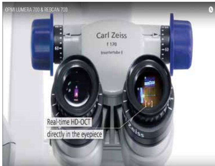
Figure 5. OPMI LUMERA & RESCAN 700 microscope, where OCT images can be observed in real time.
