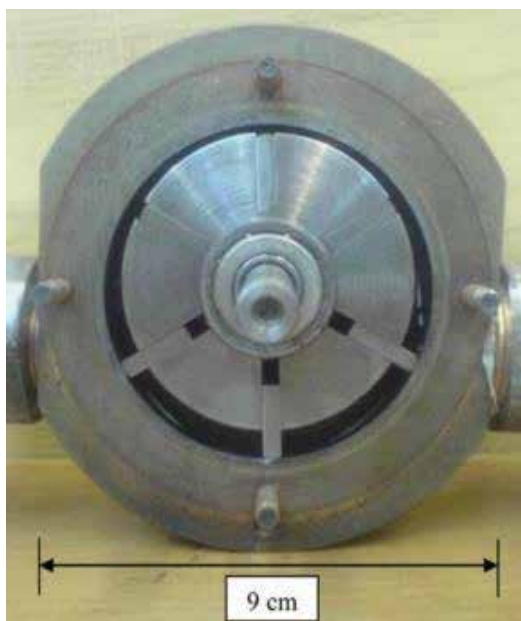
Figure 13. Photograph of the actual vane expander from the works of [20].
