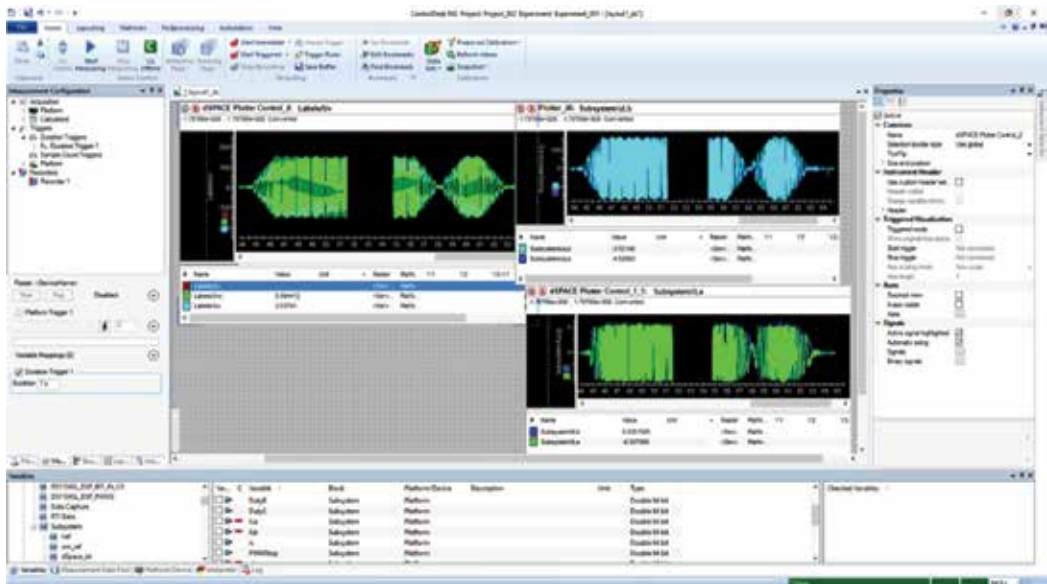
Figure 18. The ControlDesk real-time interface for controlling PMSM [9].
