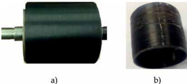
Figure 1. Rotor (a) with a rotor sleeve made of composite material (b).
