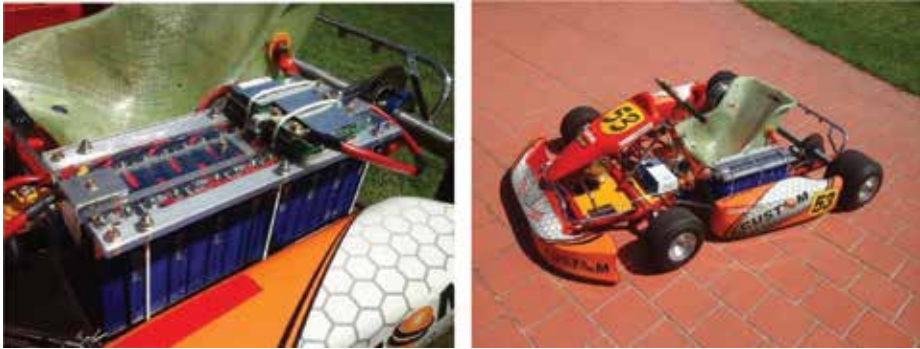
Figure 9. 48 V Lithium-ion battery pack with BMS and the prototype electric kart.
