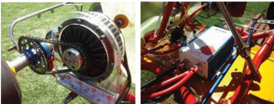
Figure 8. PMDC 10 kW motor and Q1 450 A controller.
