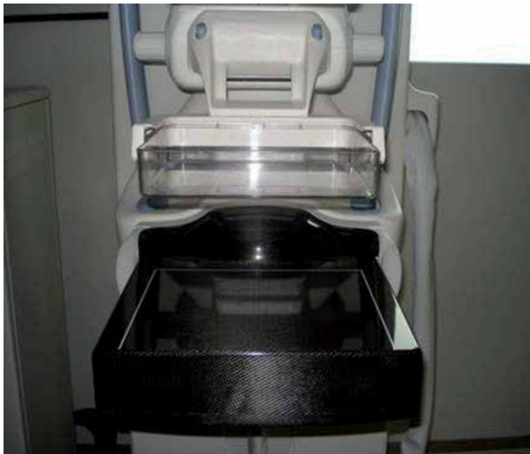
Fig. 7. Example of a FFDM detector system. Pictured is the General Electric Senographe Essential.
