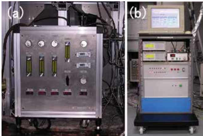
Fig. 12. Hardware of the gas control system of the HCS (a), and computer to control the gas flow together with temperature monitors and Liquid helium level meter (b).
