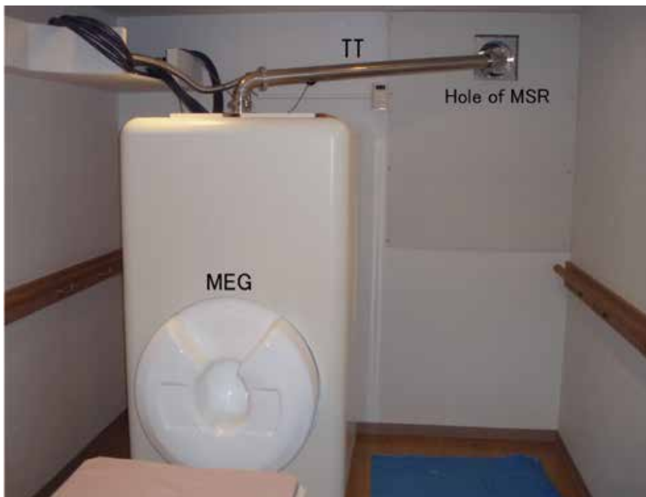
Fig. 13. Multi-pipe TT of the HCS installed on the commercialized MEG (PQ1160C, Yokokawa Electric Cor. Inc., Japan). As the TT has 1/2 inch insert tube, there was no need to modify the MEG to install the HCS. TT is twisted twice to use the ventilation hole located upper light to get through the MSR. It is tilted 5 degrees to get the LHe drop to the dewar.
