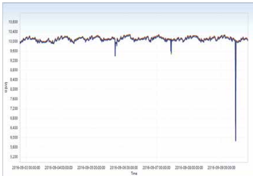
Figure 11. Voltage measurement in PCC before PV plant connection.
