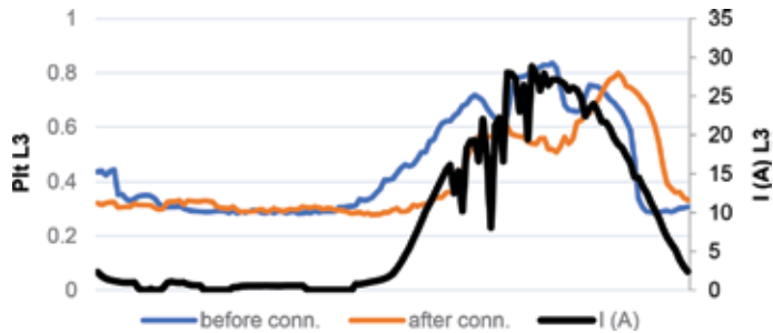
Figure 5. P_{it} L3 values before and after PV plant period regarding I_{L3} in A.
