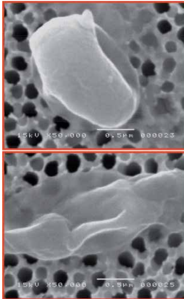
Figure 8. The impact of DIC on spore destruction is coupled thermal and mechanical (explosion) effects.
