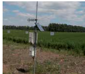
datalogger and transmitter
