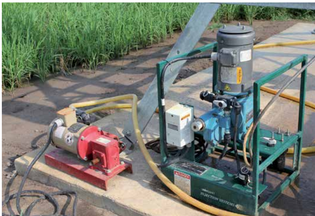
Fig. 12. Two types of injection pumps commonly used for chemigation. The pump on the left is a piston type and the pump on the right is a diaphragm type.
