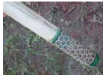
soil moisture sensor glued to PVC pipe
