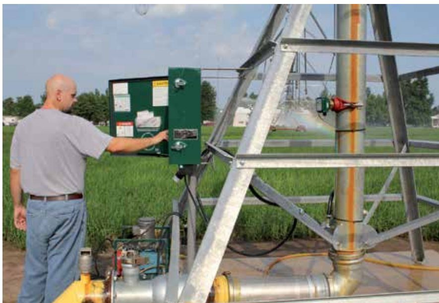
Fig. 1. Center pivot irrigation system equipped with a backflow prevention valve used to apply irrigation water, and an injection pump for applying liquid nitrogen fertilizer and fungicides for controlling diseases.
