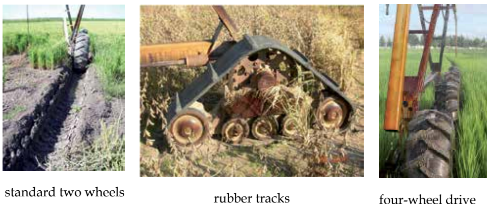
Fig. 2. Traction alternatives include (a) standard two-wheel drives, which can create deep ruts and cause the system to stall; the problem is most common on clay soils. For better flotation, (b) tracks can be added or (c) more tires used where high water flow rates occur.
