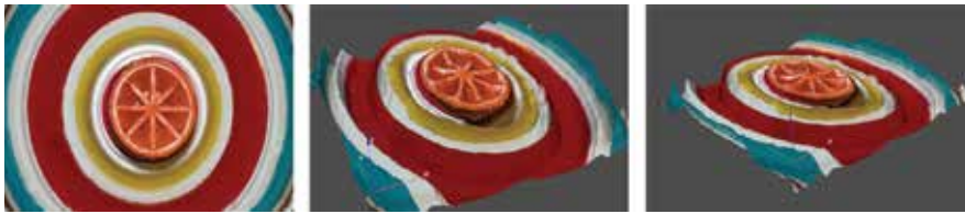
Fig. 13. Typical image that creates failed 3D model. This photograph presents a common child's spinning top. Reconstruction algorithms failed because of many smooth and uniform regions and a lack of background plane.
