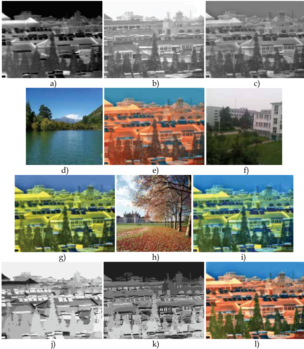
Fig. 7. Source images, reference images and fused results with different methods. (a) infrared image, (b) visible light image, (c) fusion image using gradient pyramid method, (e), (g) and (i) fusion images with global-coloring method separately using (d), (f) and (h) as reference image, (j) region map of the infrared image, (k) region map of the visible light image, (l) fused image with the region-based coloring fusion method using (d), (f) and (h) as reference images
