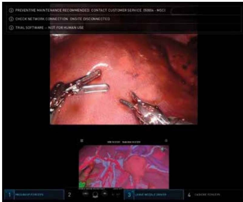
Figure 7. Real-time endoscopic overlay of 3D reconstruction over the surgical field on the da Vinci ® Xi Surgical System. The relationship between the tumor (light pink) and adjacent vasculature including the hepatic veins (light blue), hepatic arteries (red) and portal veins (blue) is present on the overlay. After initial registration, the overlay is mapped onto the patient-specific anatomy changing in real-time with camera movement.
