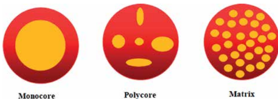
Figure 2. Schematic diagram of microcapsules model (adapted from [14]. Copyright 2009 by DESIDOC).
