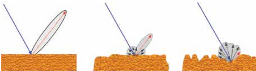
Figure 2. Scattering patterns determined by surface roughness.
