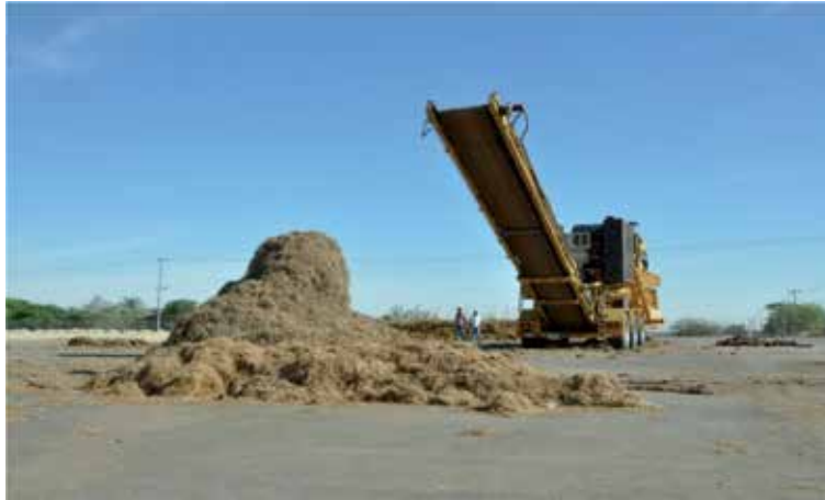
Figure 5. Shredding machine for pulverizing date palms severely infested by the red palm weevil, Rhynchophorus ferrugineus .
