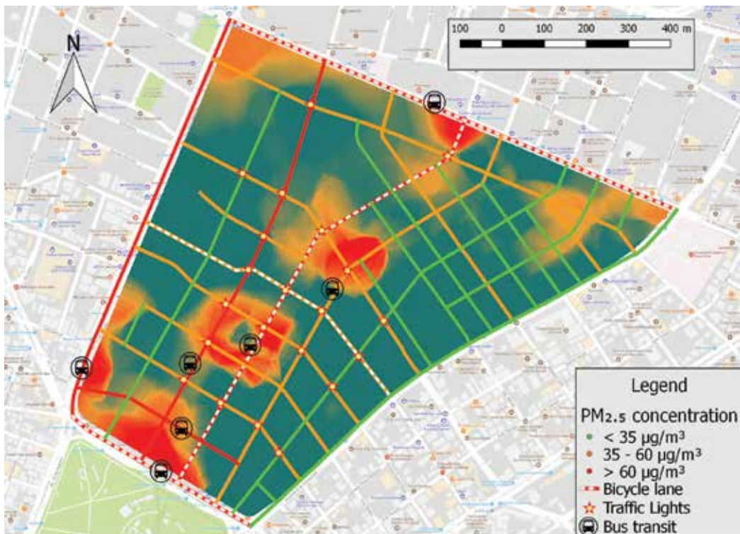
Figure 2. PM_{2.5} concentrations in the urban street network of Quito district Mariscal averaged per street and spatial interpolation (ordinary kriging).
