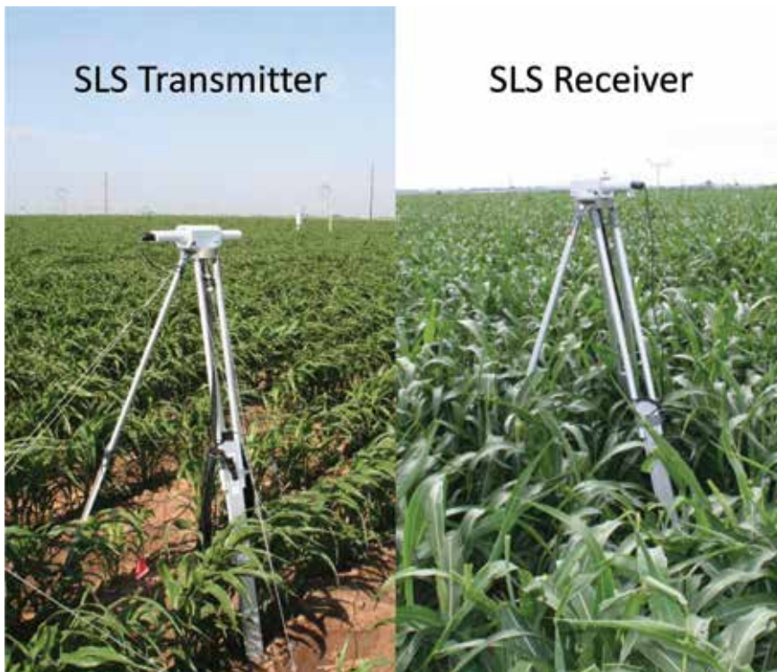
Figure 7. Surface layer scintillometer (SLS-20, Scintec AG, Rottenburg, Germany).
