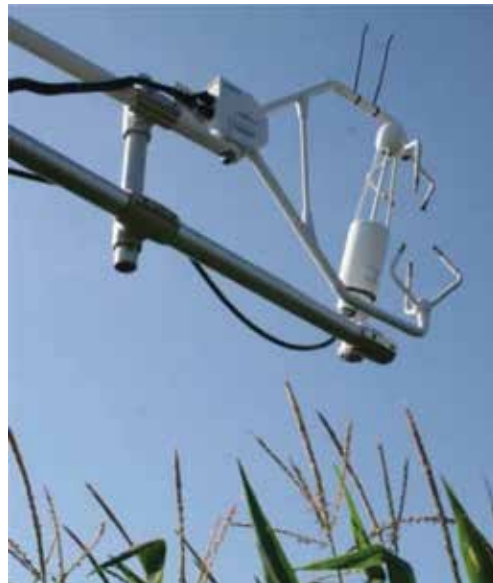
Figure 5. A typical eddy covariance system consisting of a three-dimensional sonic anemometer (CSAT-3, Campbell Scientific Inc., Logan, UT) and an infrared gas analyzer (LI-7500, LI-COR Biosciences, Lincoln, NE).
