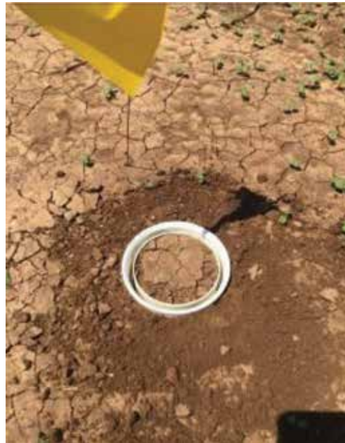
Figure 4. An example of a “micro lysimeter” used to determine soil evaporation. The inner soil container can be removed from the outer housing and manually weighed.
