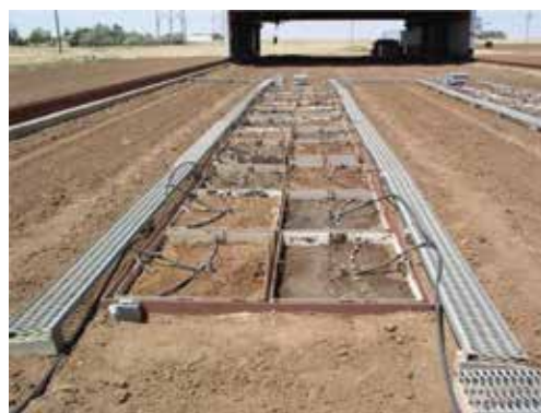
Figure 3. The Soil-Plant-Environment Research (SPER) facility at the Conservation and Production Research Laboratory (CPRL) in Bushland, TX. This facility contains 48 smaller lysimeters consisting of 12 replications of the 4 main soil types throughout the Southern Great Plains region of the United States. An automatic rainout shelter (seen in the background) covers the lysimeters during precipitation events so that water can be precisely controlled through surface drip irrigation.
