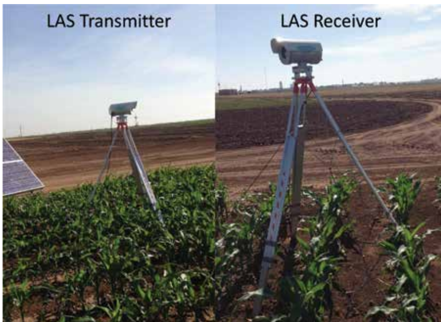
Figure 6. Large aperture scintillometer (LAS MKII, Kipp & Zonen, Delft, the Netherlands) with aperture restrictor plate reducing aperture from 15 cm to 10 cm.
