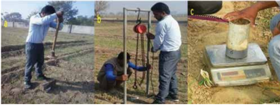
Figure 4. Demonstrating filling of lysimeters (a); pulling out filled lysimeters with specially designed chain-pulley arrangement (b); and weighting of filled and capped lysimeter (c) [28].
