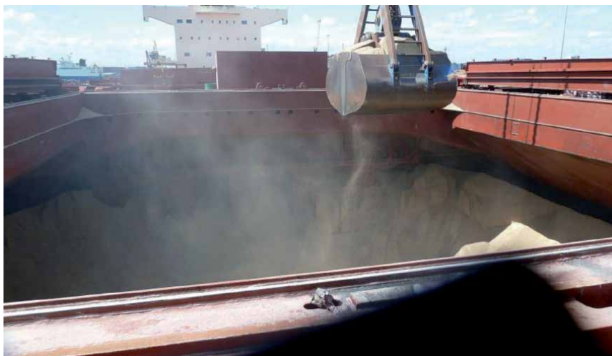
Figure 4. The crane is being used to move soya from the ship's hold to the dockside hoppers. Spillages and dust clouds from the crane's grab are noticeable.
