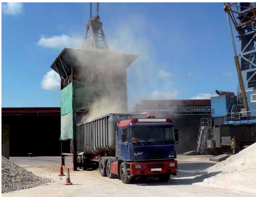
Figure 3. The visual dust cloud from a lorry loading soya from the hopper and the crane grab depositing soya into the hopper.
