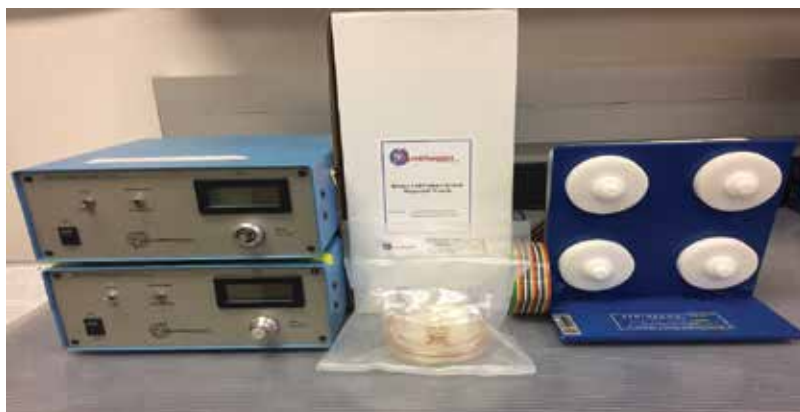
Figure 3. Rotatory cell culture system. Courtesy: OIPL lab, Texas Southern University. The RCCS was originally developed in NASA's Johnson Space Center in order to simulate the microgravity conditions of space. It is structured based on the principle of clinorotation, which is defined as the nullification of gravity's force by slowing the rotation around one or two axes. NASA's clinostat is a single axis device known as the rotating wall vessel (RWV), the RCCS is the commercial version of this device. The NASA rotating bioreactor simulates microgravity by gently moving the growth medium while growing cells are kept in suspension by a constant "free fall" effect.
