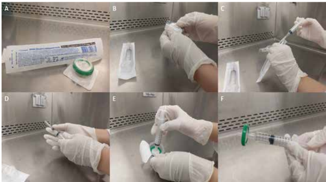
Figure 2. Step-by-step sterile air filtration in laminar flow hood. A sterile syringe that can contain 5 mL of air and a 0.2 µm filter (A) packages is opened inside a laminar flow hood (B), the syringe is carefully removed (C), the needle is detached (D), the syringe is attached to the filter (E), and 5 mL of air is loaded into the syringe (F).
