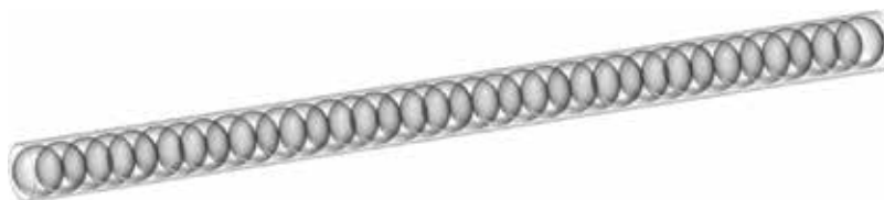
Figure 3. Schematic of series of spheres representing rod-shaped particles.
