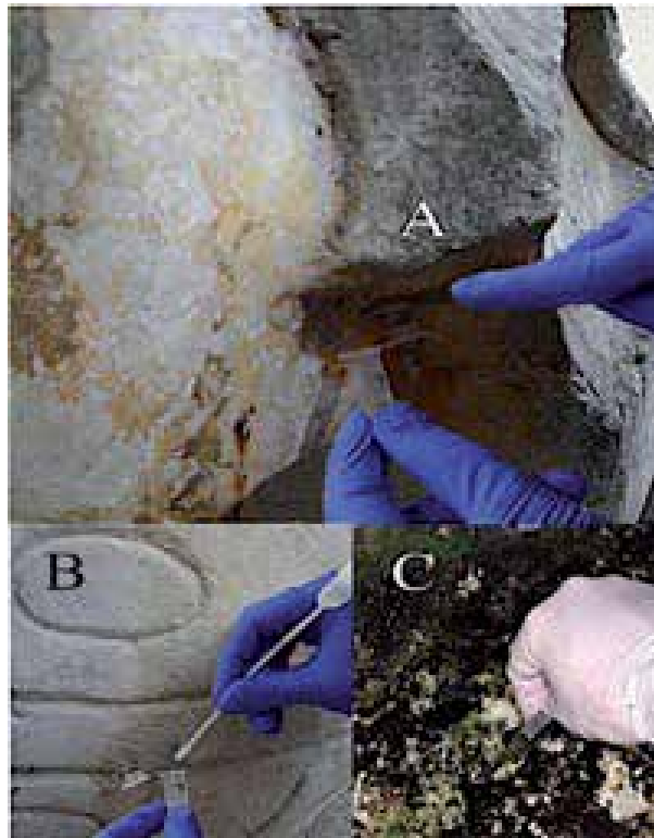
Figure 1. Stonework altered areas, sampling performed by sterile swab or scalpel: (A) dark-rust red area; (B) light – green calcareous deposit; (C) dark-green area.
